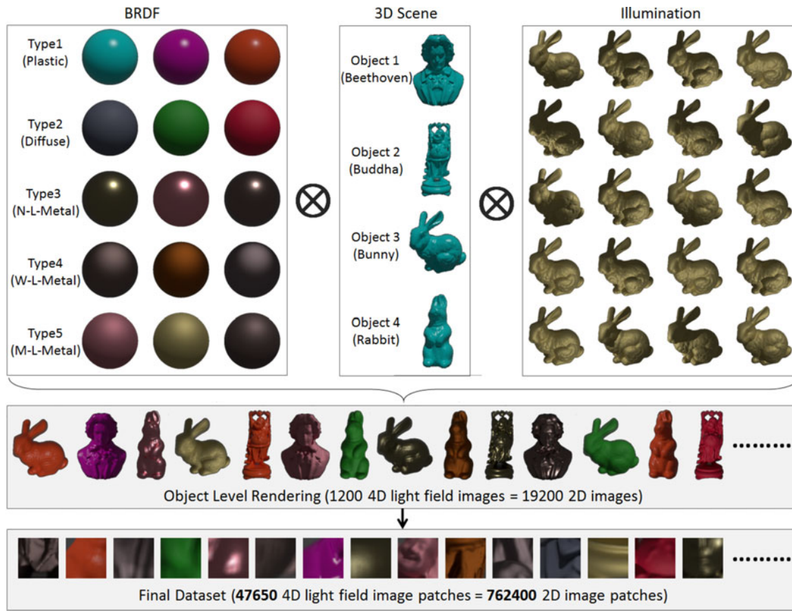
Fig. 5. The proposed dataset for the BRDF identification task. The dataset is generated via image synthesis with five typical types of BRDFs, namely, plastic, diffuse, narrow-lobe-metal, wide-lobe-metal, and mid-lobe-metal BRDFs, four typical 3D objects, namely, Beethoven, Buddha, Bunny and Rabbit, and twenty different illumination conditions. Totally 1200 4D light field images are synthesized which comprise 19200 2D images. Finally, we carefully crop out 47650 4D light field image patches (comprising 762400 2D image patches) from the images to form our dataset.
